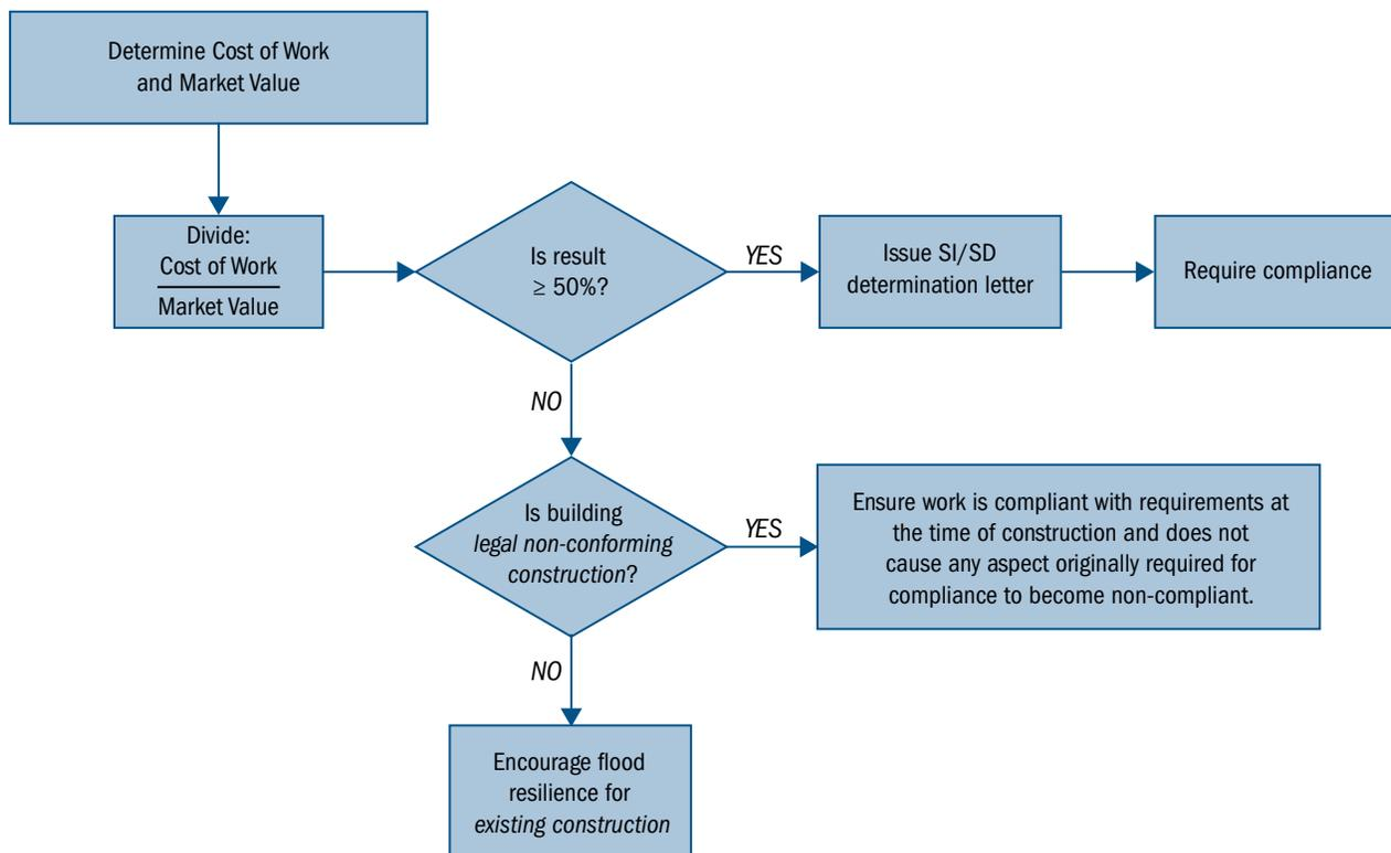
Figure 2-6. Overview of the SI/SD determination process
